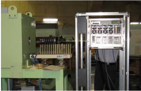
Fig.2 Photograph of the test setup. 4 CPU modules are placed behind a shiny metal grid.
